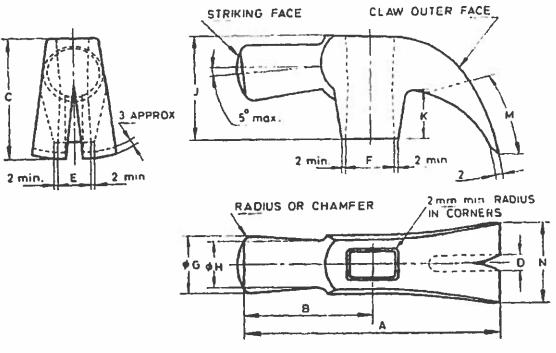
Figure 1: General arrangement of the hammer head
